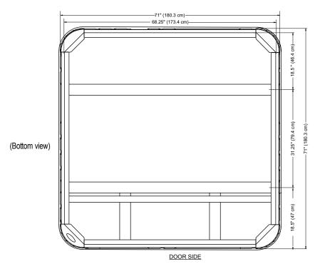
**NOTE:** Watkins Manufacturing Corporation recommends that the SX be installed on a minimum 4" (10.2cm) thick reinforced concrete pad or structurally sound deck able to support the "dead weight" found in the spa specification chart.
