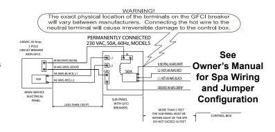
field wiring access panel of the control box. A licensed electrician should install a four-wire electrical service (two line voltages, one neutral, one ground) from the main electrical service panel to the subpanel.
