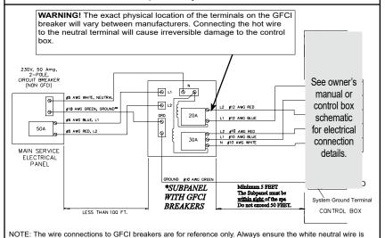
\*PROVIDED WITH SPA. NOTE: ALL WIRING SHOULD BE COPPER.
